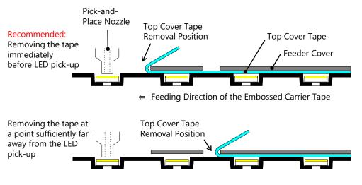
Figure 3. Top Cover Tape Removal Position
