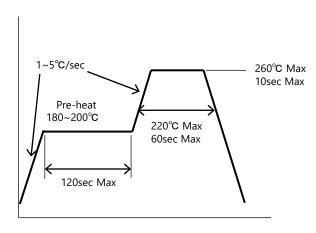
Figure 7. Recommended Reflow Soldering Condition (Lead-free Solder)
