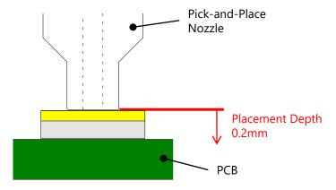
Figure 5. Recommended Nozzle Height for Placement (Placement Depth)
