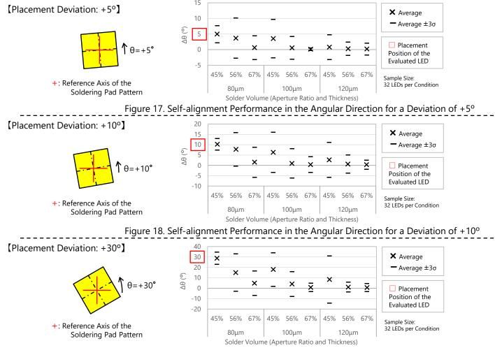
Figure 19. Self-alignment Performance in the Angular Direction for a Deviation of +30°
