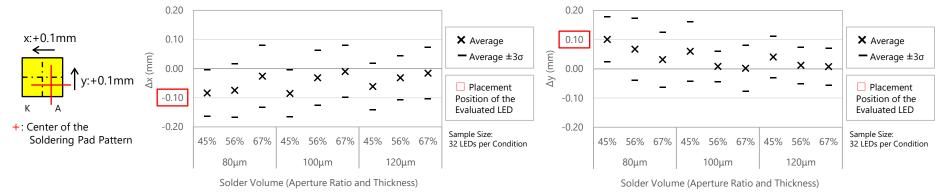
Figure 13. Self-alignment Performance in the x Direction for a Deviation of  $\pm 0.1$ mm
