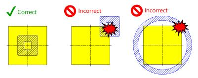
Figure 2. Correct/Incorrect Examples of LED Pick-up Positions
