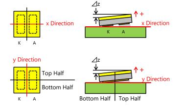
In the z-x direction, if the anode side of the LED is higher, the LED is regarded as being tilted in the plus direction; if the cathode side is higher, the LED is regarded as being tilted in the minus direction.
