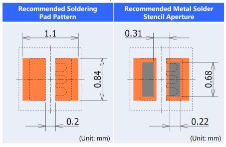
Table 4. Recommended Solder/Metal Solder Stencil Conditions
