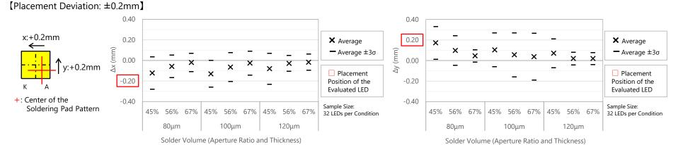
Figure 15. Self-alignment Performance in the x Direction for a Deviation of  $\pm 0.2$ mm
