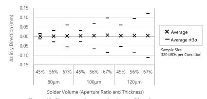
Figure 12. Placement Accuracy in the z-y Direction
