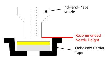
Figure 4. Recommended Nozzle Height for Pick-up Operations
