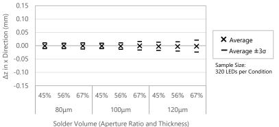
Figure 11. Placement Accuracy in the z-x Direction
