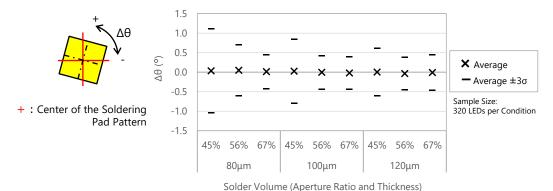
Figure 10. Placement Accuracy in the Angular Direction
